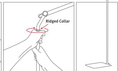
5 Attach the **iPad Clip** to the **Articulating Arm** by removing the **iPad Clip Collar** and sliding it onto the ball of the **Articulating Arm**. Firmly press the iPad Clip onto the ball of the **Articulating Arm** until it snaps into place, and then tighten the collar back onto the iPad Clip.
