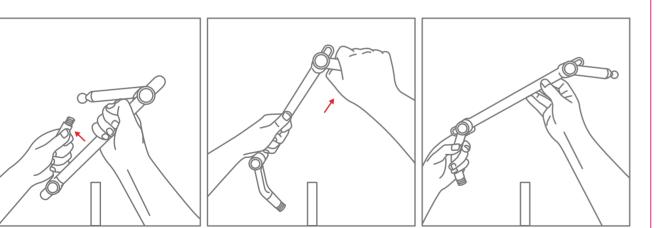
4 Attach the **Articulating Arm** to the **Tower Post** by carefully aligning the threads and screwing the **Articulating Arm** onto the **Tower Post**. Once hand-tight, give a last firm twist to the **Ridged Collar** of the **Articulating Arm**.
