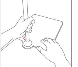
3 Unfold the **Articulating Arm** by firmly grasping the body and pull each stalk outward approximately to the positions shown below.
